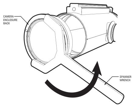
Figure 5. Remove Back Cap of Camera Enclosure
